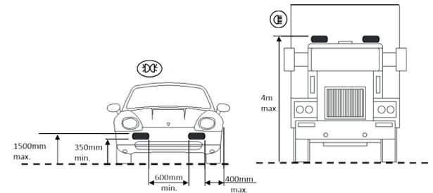
**EN** Lamps with integrated Position light may need to be positioned according to the above sketch. If an additional pair of position lights is not permitted (e.g. in Switzerland, Austria), the position light should be disconnected. The legal regulations in individual countries must be observed.
